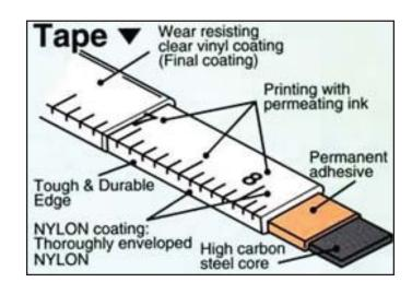
Steel tape coated with protective white nylon in ABS Open Reel.
